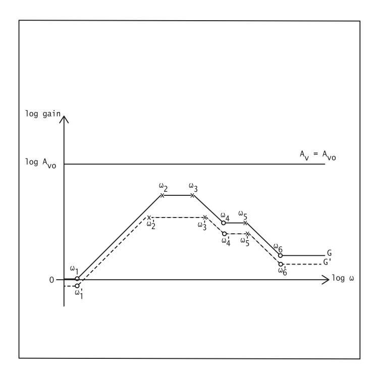
$\underline{\text{Fig. 6}}$  The effects of inadequate loop gain:
